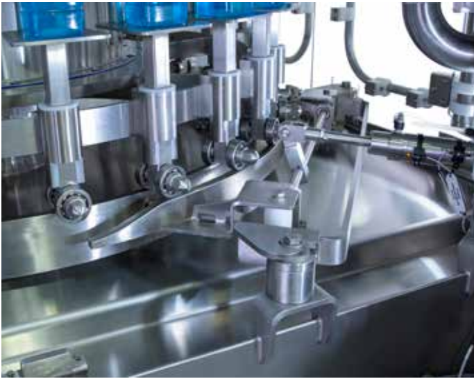
Optional automated CIP drain pan system keeps product and CIP fluids off the filler base and plant floor
