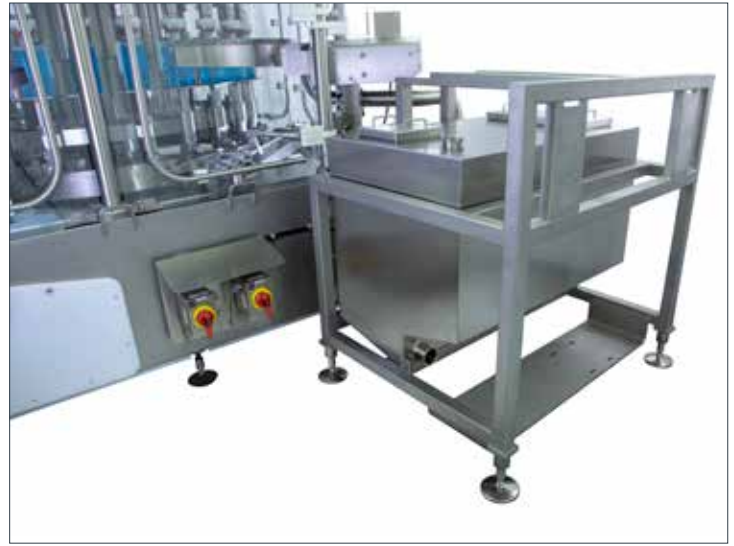
Optional externally mounted CIP fluid collection & containment tank temporarily holds drained product, CIP fluids, sanitizers and rinse fluids so they can be efficiently pumped to reclaim or reprocessing systems
